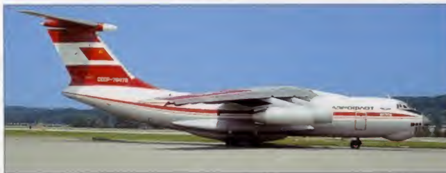
The undercarriage doors close when the wheels are down to prevent the entry of mud, snow and ice. Braking is hydraulic and the tyre pressure can be altered from the cabin. Two packs of 96 50-mm (1.97-in) flares can be carried on the landing gear fairings and a further two on each fuselage side.
